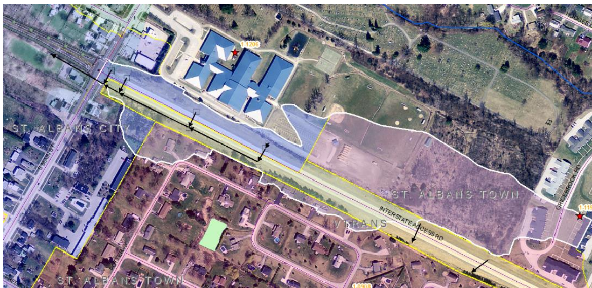
Figure 20: Drainage area for SASH/Route 7 culvert, with MS4 boundaries. The proposed plan as of January 2015 for the Nason St. Connector road was included in this map (NW corner).
